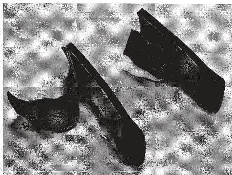
Figure 6. Specimens to test adhesion between inner and outer layers (peeling).
